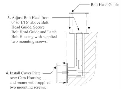
**Note:** If prepped holes are not perpendicular cam housing may bind. Break edge of the intersection of the 2 holes or file the edge of the vertical hold to ensure the noted dimension.
