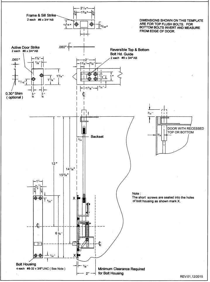
SCREW DETAILS: #8-32 x 3/8" UNC - flat countersunk head machine screw, total 4 pcs.
