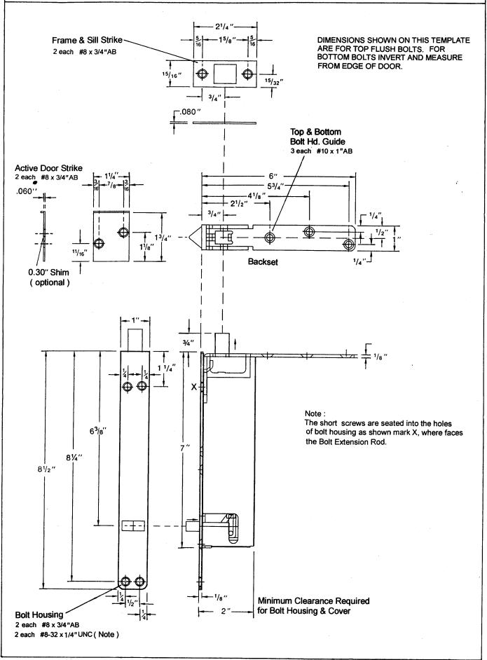
SCREW DETAILS: #8-32 x 1/4" UNC - flat countersunk head machine screw, total 2 pcs.
